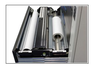
5. Insert the leading edge of media under the feeding roller.
