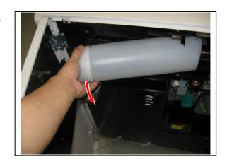
5. Shake the new Toner Cartridge fully to loosen the toner.
