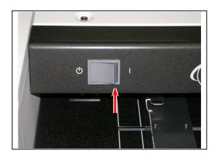
3. KIP 9900 starts warming up the Fuser Unit, and the Ready Indicator on the Operation Panel starts flashing.
