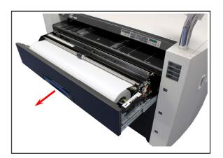
2. Rewind the roll media to release the leading edge from feeding rollers.
