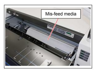
6. The leading edge of roll media is still in the Cutter Unit as the following section drawing. As this state will result in another mis-feed, the media needs to be rewound. Draw out the concerning Roll Deck and rewind its roll media.
