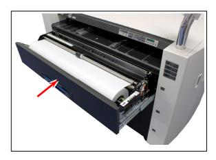
6. Select the concerning Roll pressing the SELECT Key, and press the CUT Key to take Initial Cut.
